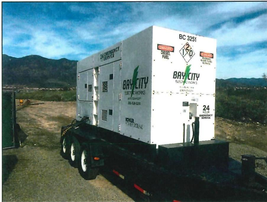
Temporary Generator used for Testing
